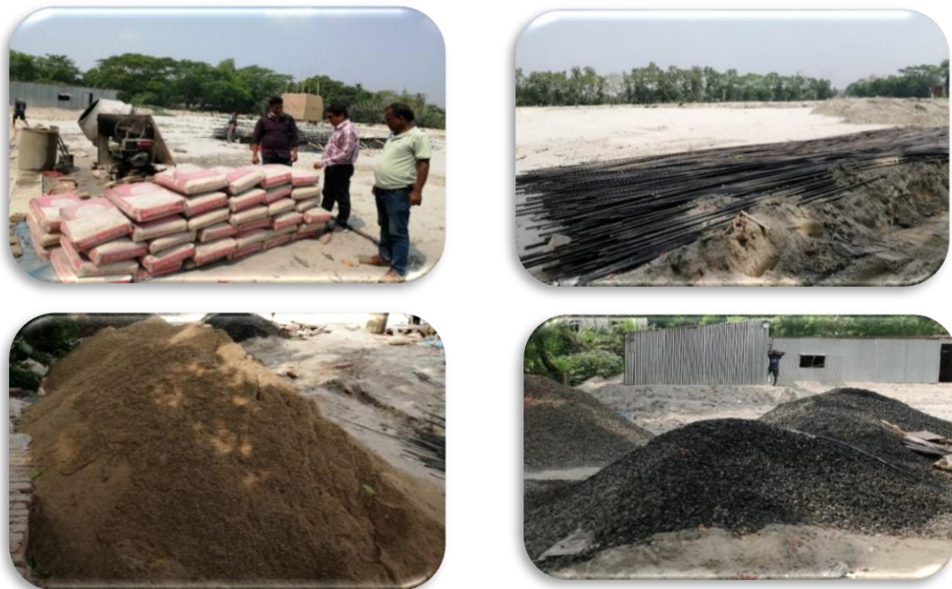
Image 3.9 Cement (King Brand), Rod (SS Tiger 400 DWR 60 Grade 20/16/10 mm), Sand (Sylhet St) and Stone Chips (as per specification) – starting from top left ( clockwise)
